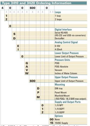
\* Type 3400 DeviceNet "D" mounting, Type 3400S and DeviceNet board installed in a single extended DIN tray. 'P' or 'M' mounting, DeviceNet board is supplied with 4 screws and stand-offs for panel mounting.
