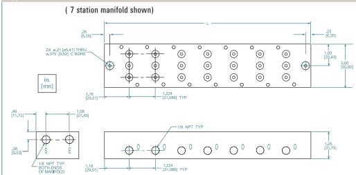
Manifolds are available in 2 to 10 stations. To calculate the overall length "L" of the manifold use the following formula:
